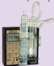
Impinger and trap in holder mounted on Universal Deluxe Sample Pump
