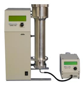
Real-time particle number size distribution measurement system and monodisperse particle generator
